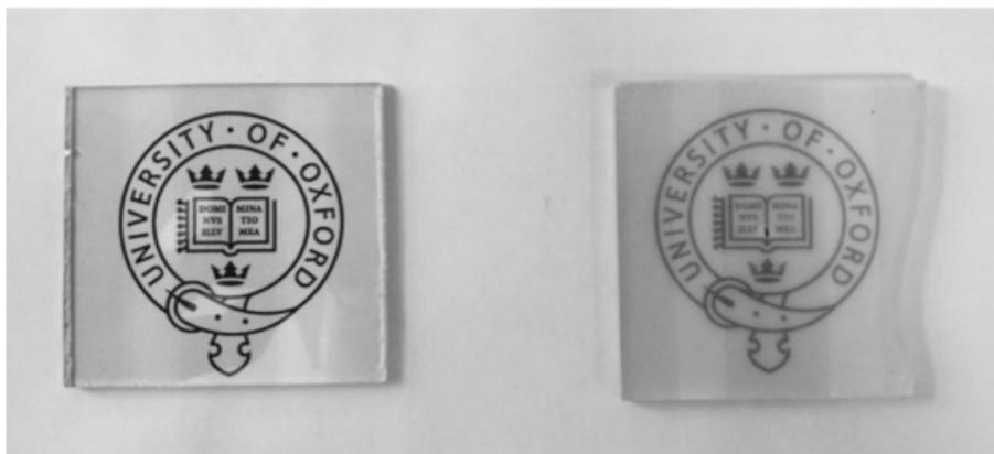
Figure 6.2: (Left) flat TiO<sub>2</sub> film on an FTO substrate; (Right) macroporous TiO<sub>2</sub> film.
